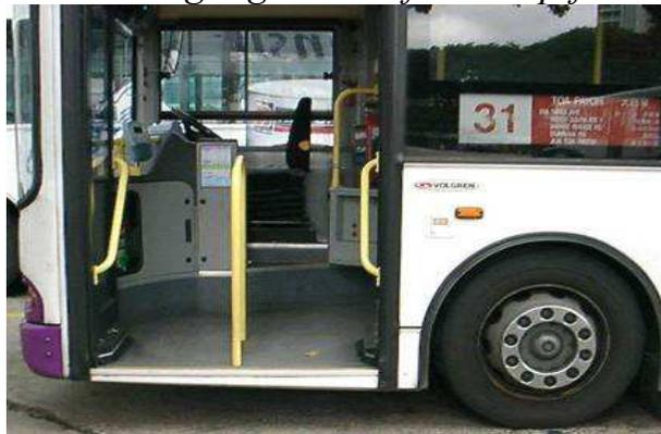
A low-floor step-free bus has a lower gap between the bus floor and road kerb.
